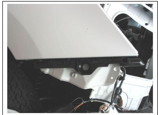
Figure 6 - Remove plastic bumper support from under guard.
