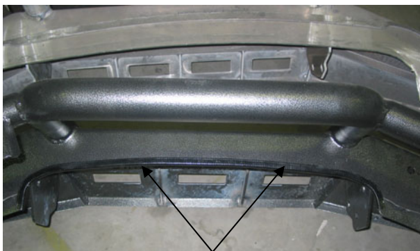
Attach 6mm clip lock trim Note: Non winch bar shown
